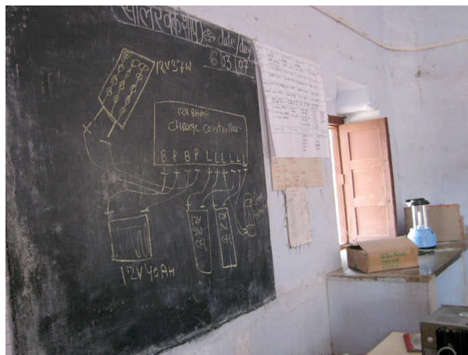
Circuit diagrams for a solar lantern
