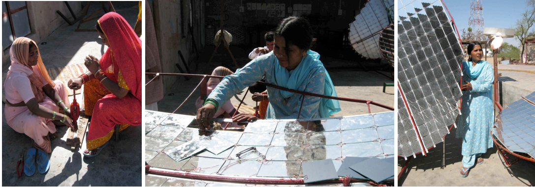
From drilling holes in the mirrors, to assembling sun tracking mechanisms on solar cookers
